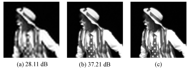
Fig. 3. Details of the results for the Pantomime view 39, frame 0. (a) Downsampled and upsampled by 4 with a Lanczos filter. (b) Downsampled by 4 and super-resolved with a Lanczos filter, using two full-resolution views. (c) Original. Results are best seen on a screen.
