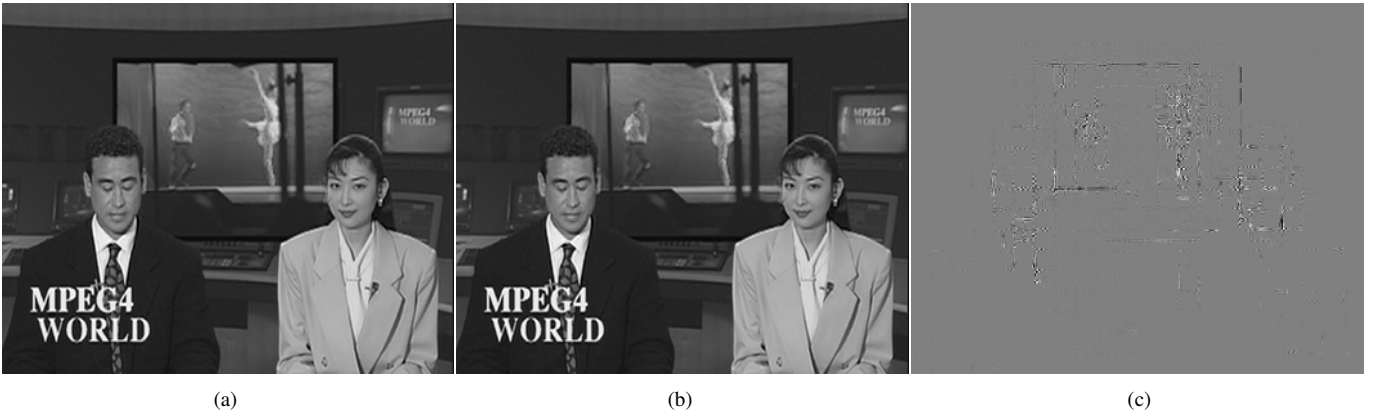
Fig. 12. SR results of the 16th frame of the News sequence: (a) using OBMC and (b) regular block-based motion compensation. (c) Difference between (a) and (b).
