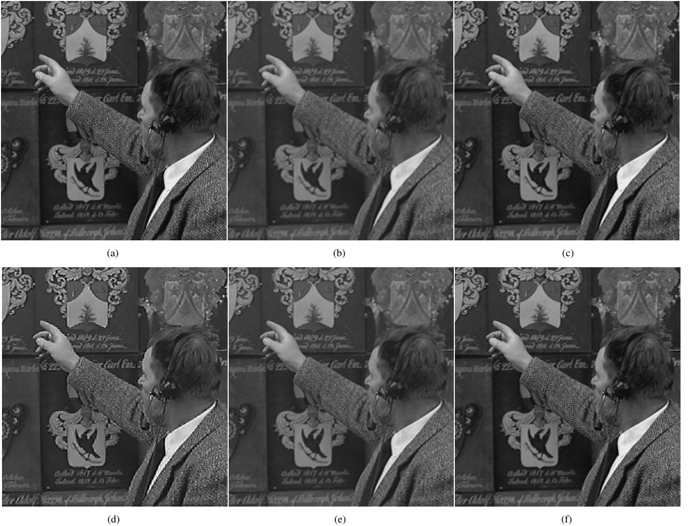
Fig. 15. A region of the 16th frame of sequence Shields: (a)original, (b) interpolated with Bicubic filter, (c) interpolated with Lanczos filter, (d) super-resolved with [11] (e) super-resolved with [13] and (f) super-resolved with the proposed methods.
