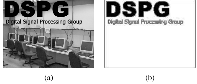
Figure 2. Classification algorithm: (a) original grayscale image (2592x1952 pels); (b) its coding map.
