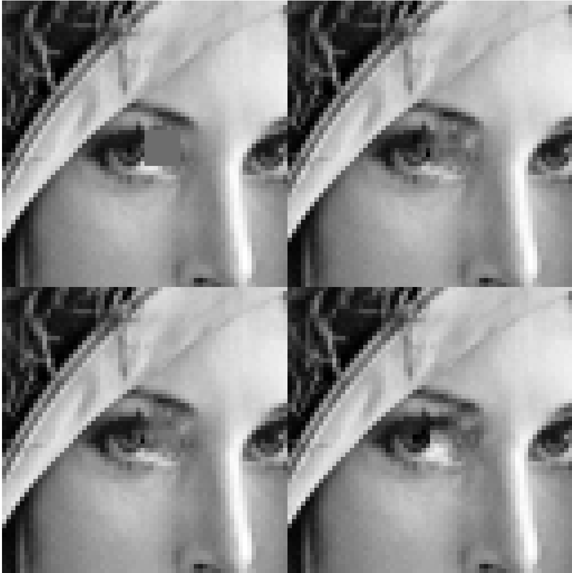
Figure A.7: Trivial image reconstruction when all AC coefficients of a single block are lost. The AC coefficients are set to zero in this block and a zoom of reconstructed images for each transform are shown. Top left corner, DCT. Top right corner, LOT. Bottom left corner, LOT-2. Bottom right corner, ELT-2.
