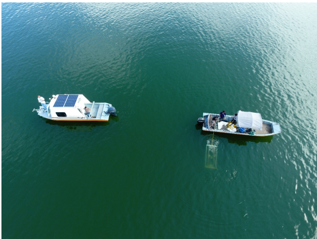
Fig. 4. Image of the installation of the target at one of the acquisition sites, showing the support vessel (right) and acquisition vessel (left).
