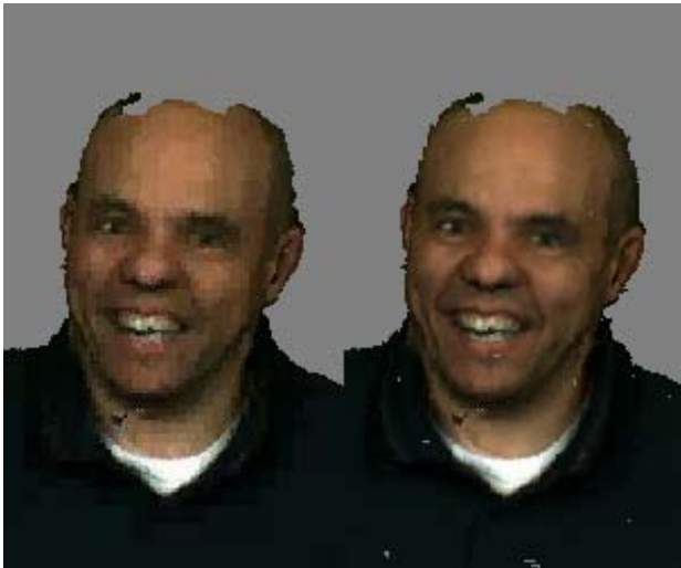
Fig. 13. Front projection rendering comparing MCIC (correspondence-based distortion) on the right against intra-coder (RAHT) on the left, for frame 60 in sequence “Ricardo,” both encoded at about 2.6 bpv.
