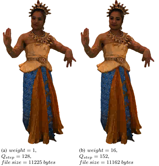
Fig. 4. Point cloud Thaidancer ( N_{vox} = 689953 ) coded with different weights for voxels in the ROI. The Q_{step} was adjusted to result in similar file sizes.
