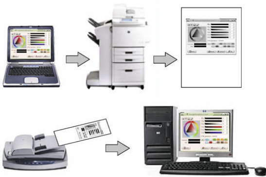
Fig. 1. Illustration of the color to gray conversion application. The color image is printed in a black and white printer. Later on, the user may scan the printed document and recover the original colors, if so desired.
