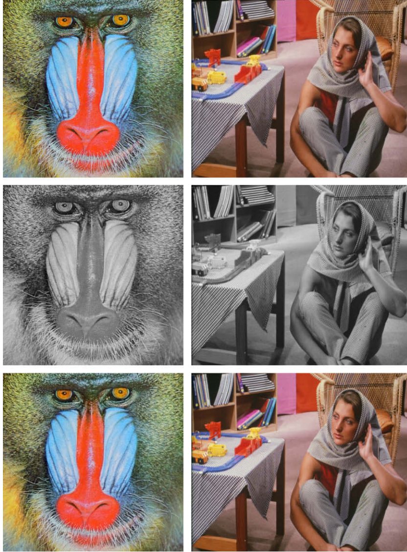
Fig. 8. (Top) Original color images “mandrill” and “Barbara”, (middle) their respective texturized grey versions, (bottom) and the recovered color images without printing by scanning, or any other noise. In essence the bottom images are recovered directly from those in the middle row.
