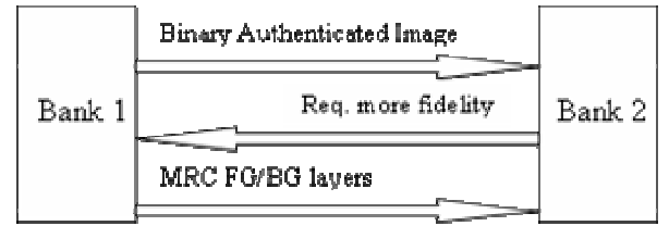
Figure 1. Proposed framework for check exchange. First the BW image is sent, and, if necessary, the foreground and background layers are also sent.
