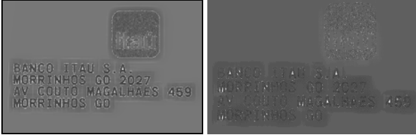
Figure 7. Halo around the text makes the image more difficult to compress. Left: unprocessed; right: pre-processed.
